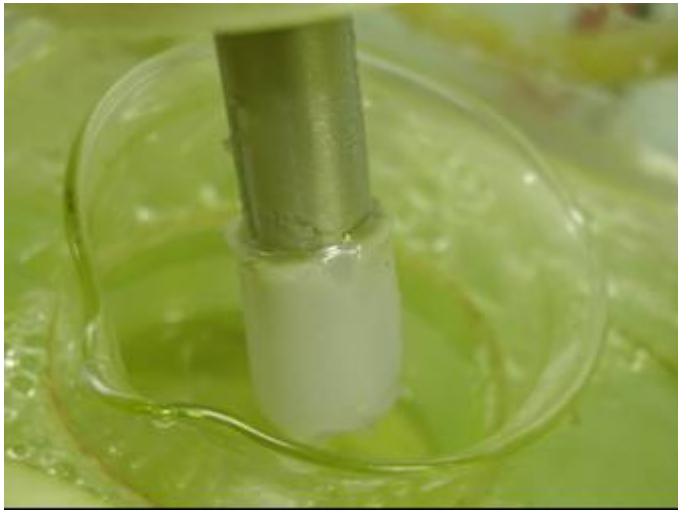
Figure 2: Cold Finger Deposit - Lubsnap 40 – 2.2% Wax
