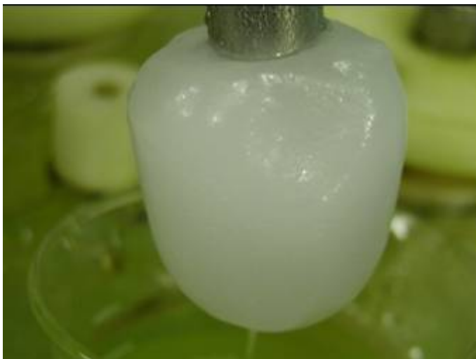
Figure 3: Cold Finger Deposit - Lubsnap 40 – 5% Wax
